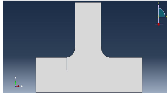
Figure 2. T-butt weld with (a) vertical crack
